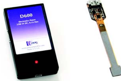
DigiTacts 2x2 Sensor Array with D600 Interface Module
